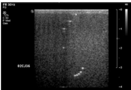
**Figure 5.** Transducer uniformity rating = "4." Sufficient damage exists to replace the transducer. This transducer was taken out of service immediately after QA testing.
