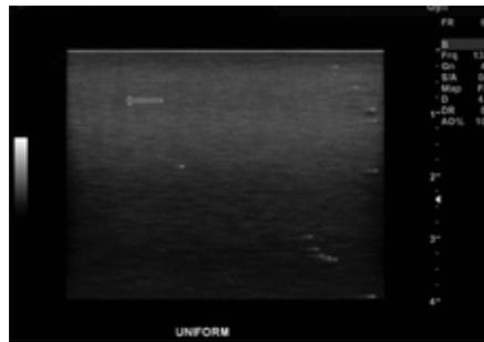
**Figure 3.** Transducer uniformity rating = "2." One or 2 minor nonuniformities are present; generally, the transducer is classified as "watch and wait" and is still usable. (From *AIUM Quality Assurance Manual for Gray Scale Ultrasound Scanners.*)
